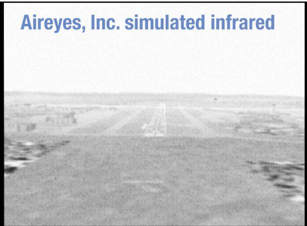
CATII DAYTIME FOG CONDITIONS, AT APPROXIMATELY 100' AGL. RUNWAY THRESHOLD IS BARELY VISIBLE IN LEFT PANEL (SIMULATOR VISUAL). SUN-IRRADIATED FOG LEADS TO BRIGHT SKY IN INFRARED (RIGHT PANEL). INFRARED SENSOR DEGRADATION IN ALL TYPES OF WEATHER CAN BE CUSTOMIZED AND CALIBRATED TO MATCH ACTUAL PERFORMANCE OF SPECIFIC INFRARED SENSORS (DETECTOR, OPTICS, PROCESSING).
